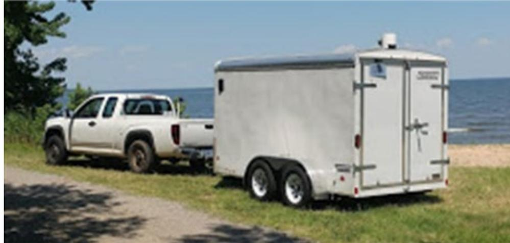
Wind profiles from about 100 m to ~3000 m or more (depending on atmospheric conditions and lidar settings) at ~1 km horizontal spacing and 30 m vertical spacing.
